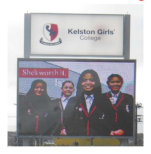
Two signs (one each side) full colour 10mm pitch 1760mm (H) X 2400mm (W) mounted on existing structure to replace old LED sign. New light box with school logo placed above.
