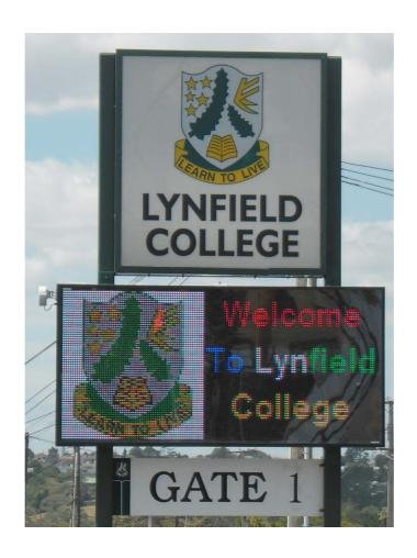
Two signs (one each side) full colour 16mm pitch 1024mm (H) X 2304mm (W) mounted on existing structure to replace letter board.
