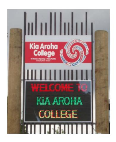
Tri- colour 20mm pitch 640mm (H) X 1920mm (W) on double timber poles with static signboard on timber grid above.
