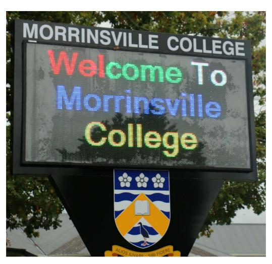
Full colour 10mm pitch 800mm (H) X 1760mm (W) on Single post with static signboard above.
